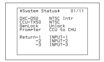
**DXC-D50:** Model name and format of the connected camera
